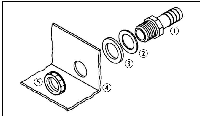
**8** Condensate Drain Installation for Other Self-Contained Systems
