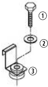
**9** Mounting Bracket Installation for Turbo Systems
